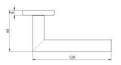
Lever on concealed fix press on round rose. Straight round bar lever neatly mitred where it adjoins the stem. Part of the range in grade 304 Stainless Steel. Comes with a 10 year mechanical guarantee and is Fire Door Rated.
