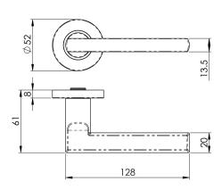
Lever on concealed fix press on round rose. A straight smooth round bar lever on rose. Part of the Grade 304 stainless steel range. Comes with a 10 year mechanical guarantee and is Fire door rated.
