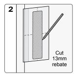
Wood Cutout: Remove middle section of flush pull template, position for desired backset and mark cutout outline. Use midline as height reference. Cut 13mm rebate
