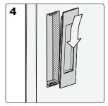
Insert flush pull into cavity. Push in and down so it grips onto the bottom bracket or edge.
