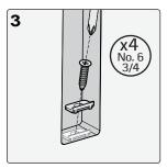
For wooden doors: install two woodfix brackets at top and bottom of cutout on both sides of the door.
