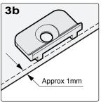
Fix brackets in centre of the cutout with the ridge facing outwards. Ensure that they are approx 1mm inside the edge and do not protrude.
