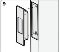
Insert end pull into cavity. Push in and down so it grips onto the bottom bracket or edge.
