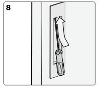
Use Mardeco hex tool to tighten grub screw inside top of flush pull. Ensure it is fitted firmly.
