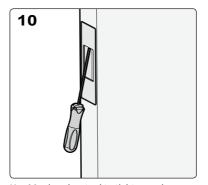
Use Mardeco hex tool to tighten grub screw inside top of end pull. Ensure end pull is fitted firmly.
