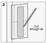
Wood Cutout: Remove middle section of flush pull template, position for desired backset and mark cutout outline. Use midline as height reference. Cut through all.
