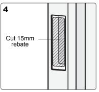
Place middle section of end pull template into rebate and mark 2nd rebate outline. Ensure it is the correct way up. Cut 15mm rebate
