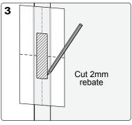
Remove middle section of end pull template and mark rebate outline on end of door. Use midline as height reference. Cut 2mm rebate.
